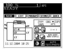
4 Choose the desired image type mode by pressing one of the PHOTO, TEXT, and TEXT/PHOTO keys.
